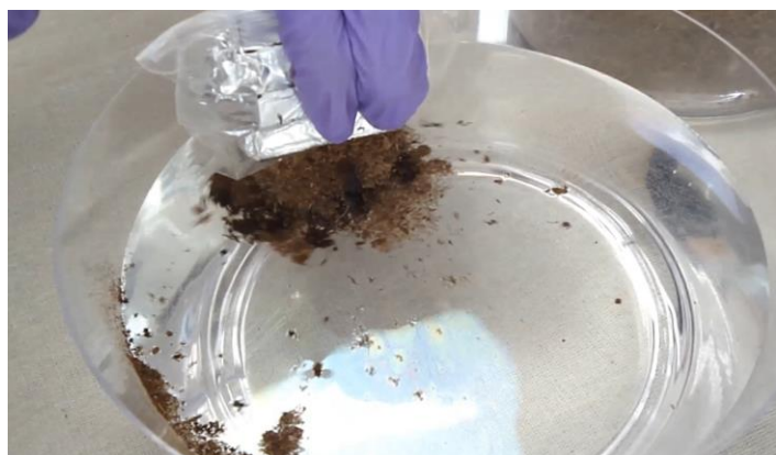
Magnetic retrieval of oil and magnetizable absorbent
