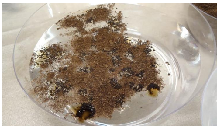
Oil and magnetizable absorbent in water
