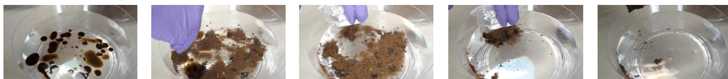
Spilled oil is absorbed by MAT and lifted by a magnet
