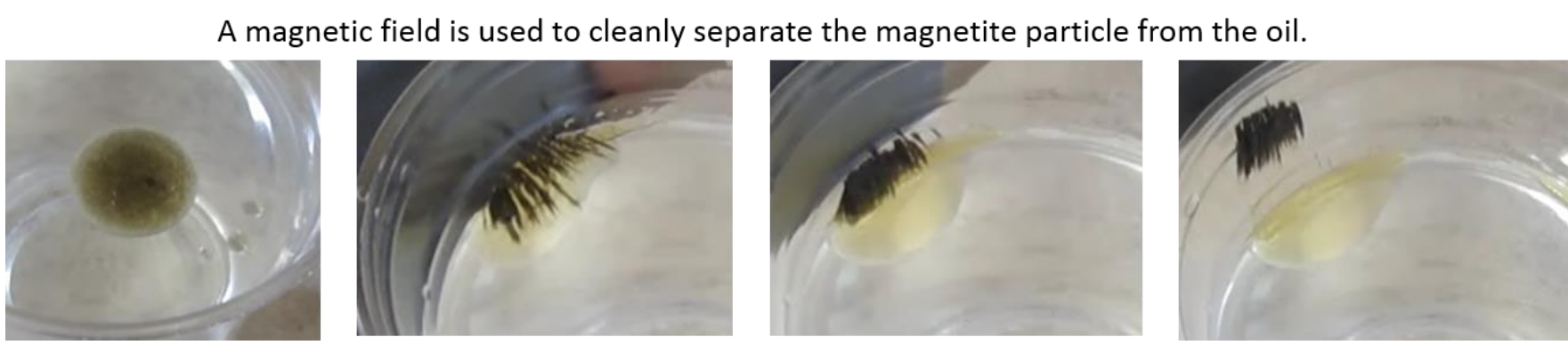
Sequence of images illustrating the magnetic separation of the magnetite particles from the oil using a permanent magnet.
